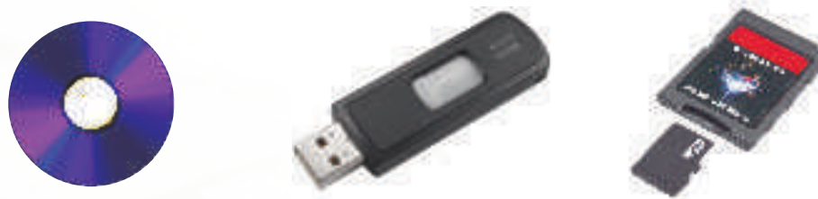
Figure 1.13 Secondary Storage Devices
