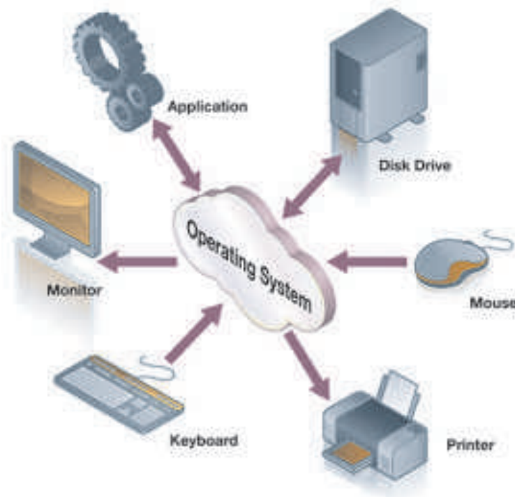
Figure 2.5 Components controlled by an Operating System
