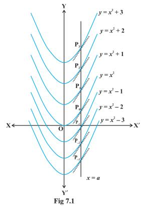
the tangents to all the curves  $y = F_C(x)$ ,  $C \in \mathbb{R}$ , at the points of intersection of the curves by the line x = a,  $(a \in \mathbb{R})$ , are parallel.
