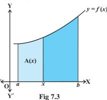
in Fig 7.3 [Here it is assumed that f(x) > 0 for  $x \in [a, b]$ , the assertion made below is equally true for other functions as well]. The area of this shaded region depends upon the value of x.
